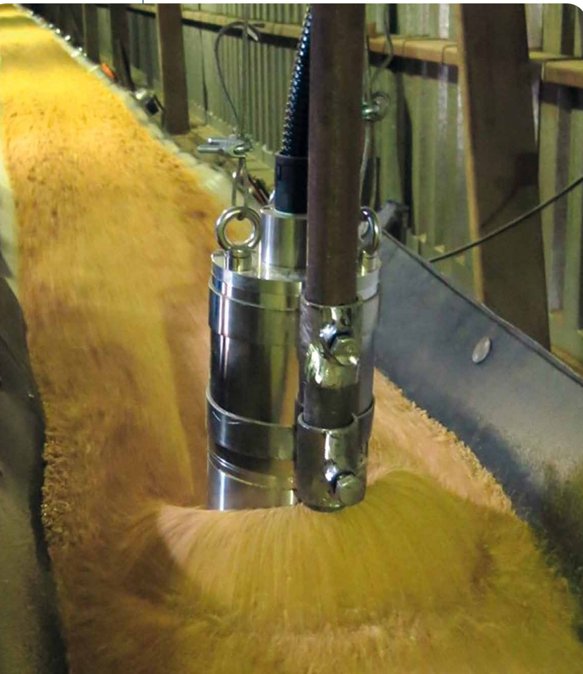
Sensor head mounted over a conveyor belt for the continuous analysis of soybean meal.
