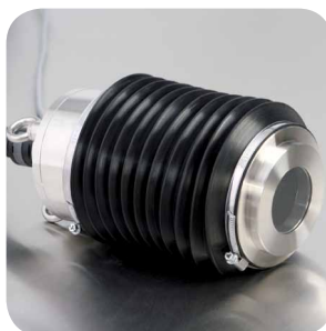
Flexible connection of the sensor head with rubber gaiter and viewing window installed, to keep the measurement area clean from dust and dirt.
