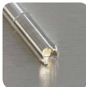
Diamond ATR fiber probe (Ø 6 mm) with protective metal tips, also for use in ATEX areas.
