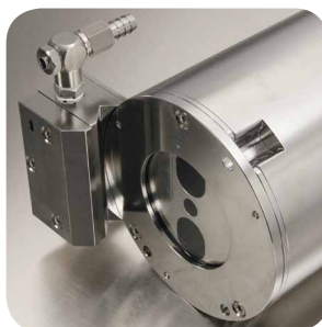
An optional air blower prevents fouling of the measurement window, e.g. by the electrostatic attraction of dust.
