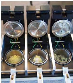
The Micro-Chamber/Thermal Extractor is a valuable tool in this regard, allowing profiles to be sampled side-by-side under identical conditions. The sensitivity enhancement of this dynamic headspace technique is raised further by combining it with TD, making it a powerful technique when trace-level aroma-active compounds are under scrutiny.
