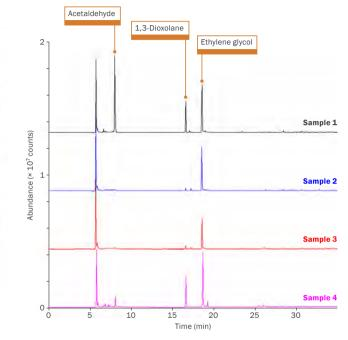
**Direct desorption** is a convenient way of comparing similar samples in order to troubleshoot taint. 1,3-Dioxolane and acetaldehyde are clear issues in two of these samples of PET (a polymer widely used in plastic drinks bottles).
