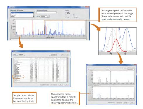
As shown in this example of bacon headspace, TargetView's interactive chromatogram (top left) allows you to delve into the results as much as you want – from a simple 'yes/no' confirmation that a particular compound is present, to detailed examination of elution profiles or comparison of mass spectra.
