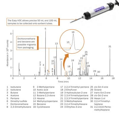
**Rapid and representative sampling of meat headspace** was achieved here using Markes' Easy-VOC grab-sampler. Packing the TD tubes with two hydrophobic sorbents allowed over 30 components to be analysed without interference from water. Removal of baseline interference and compound identification was carried out using TargetView software – see page 42.
