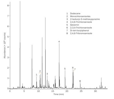
**Despite being at the sub-ppb level**, a range of commonly-encountered odorants are easily detected in drinking water using the ability of sorptive extraction with TD to enhance the concentration of semi-volatiles.
