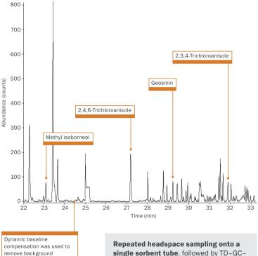
single sorbent tube, followed by TD-GC-MS analysis, is used to enhance the sensitivity for key odorants in this sample of drinking water to the low-ppt level.
