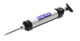
The Easy-VOC grab-sampler, with sorbent tube attached ready for sampling.
