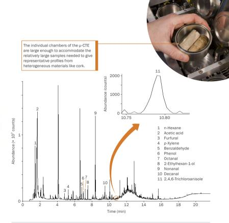
An elevated temperature was used to rapidly release the headspace from whole corks using the Micro-Chamber/Thermal Extractor ( $\mu$ -CTE), leading to the detection of TCA at trace levels despite a complex background.
